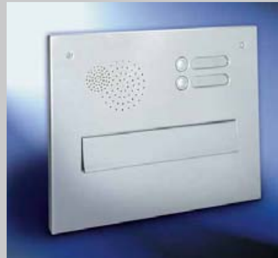
Fig. 27/4 Box format 300 x 110 x 265 - 410 mm, hinged V4A stainless steel front plate, with RSA . Letter plate 265 x 33 mm.
