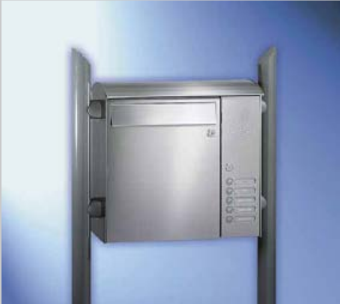
Fig. 5/1 Mail box of Model Group 10, with RSA and RS50 . CONVEX roof, side sheet casing manufactured from V4A stainless steel, 60 mm bevelled steel tubular stand. Door opening to the left, 2-point locking.
