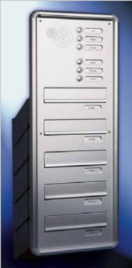
Fig. 26/1 Box format 260 x 110 x 265 - 410 mm, hinged aluminium front plate, with RSA and RS1001 aluminium radius-profile closing frame. Letter plates 230 x 33 mm.
