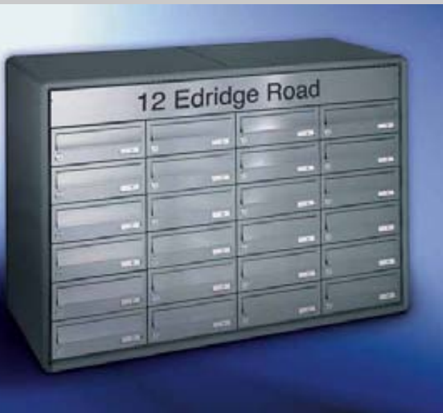
Fig. 18/1 Box format 300 x 110 x 385 mm, with RSA , inscription box and RS4000 radius aluminium casing. Letter plates 265 x 33 mm.
