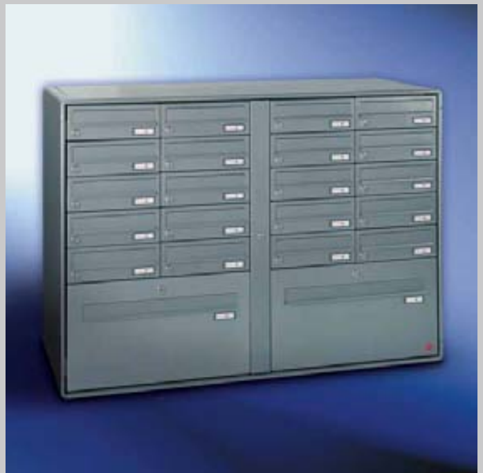
Fig. 38/4 Box format 300 x 110 x 385 mm and 2 special size boxes below, aluminium radius-profile main door frame. Front of the unit opens with 2 doors to allow mail to be inserted which is removed by the mail recipient having an individual key.
