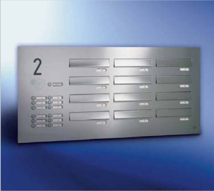
Fig. 23/1 Box format 300 x 110 x 385 mm, 24 mm front plate, with thermal break for mounting in door profile, with RSA , completely manufactured from V4A stainless steel. Letter plates 265 x 33 mm.
