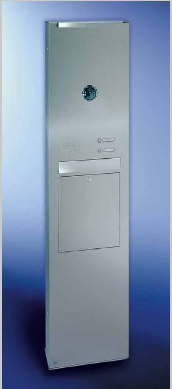
Fig. 29/2 V4A stainless steel pillar shaped mail box, one-part mail box unit with RSA , inclined opening 335 x 50 mm, box size 335 x 770 x 140 mm, front mail removal door 335 x 440 mm bottom hung with two opening restrictors, fitted with LED lighting and CCTV camera supplied by others, pillar height 2000 mm.
