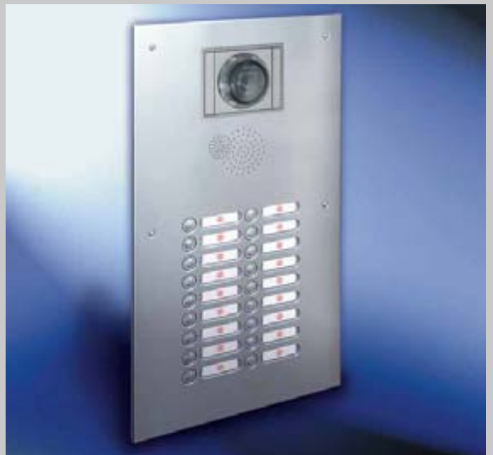
Fig. 32/4 Bespoke bell and intercom box, hinged V4A stainless steel front plate with RSA and mounting frame for CCTV camera etc. supplied by others.
