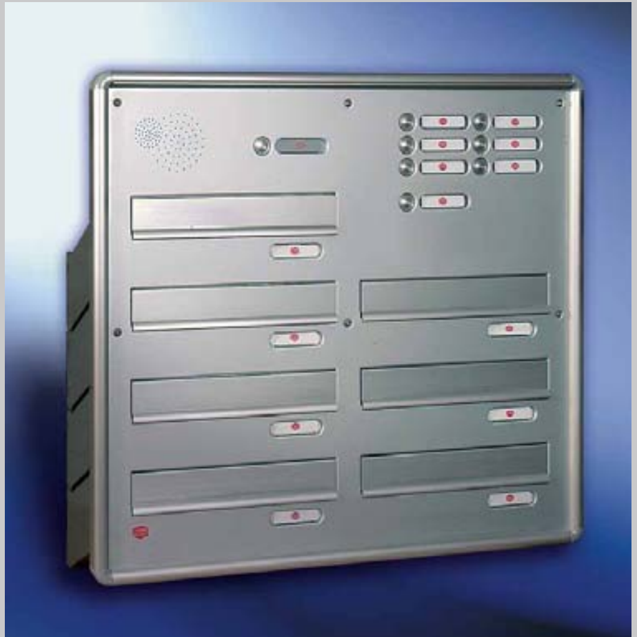
Fig. 26/2 Box format 300 x 110 x 265 - 410 mm, hinged aluminium front plate, with RSA and RS1001 aluminium radius-profile closing frame. Letter plates 265 x 33 mm.
