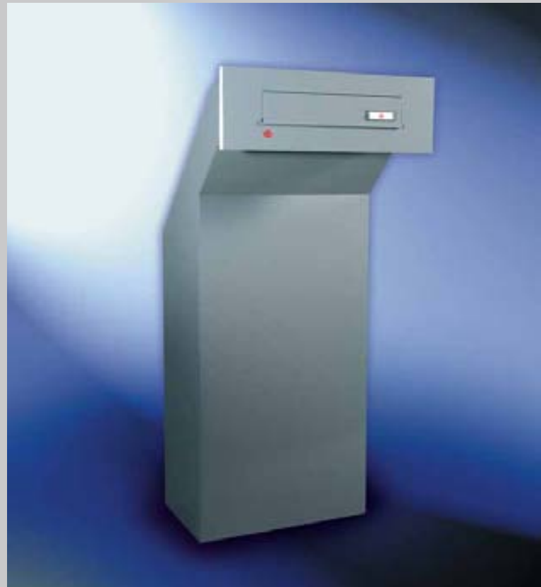
Fig. 5/4 Mail box unit from Model Group 12, box with angled chute adjustable in length for different wall thicknesses and fitted with a flush mounted mail removal door, front thermally broken.
