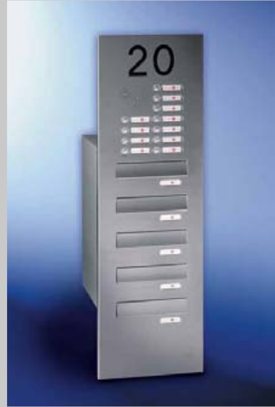
Fig. 23/2 Box format 260 x 110 mm x 385 mm, 24 mm front plate, with thermal break for mounting in door profile, with RSA , completely manufactured from V4A stainless steel. Letter plates 230 x 33 mm.
