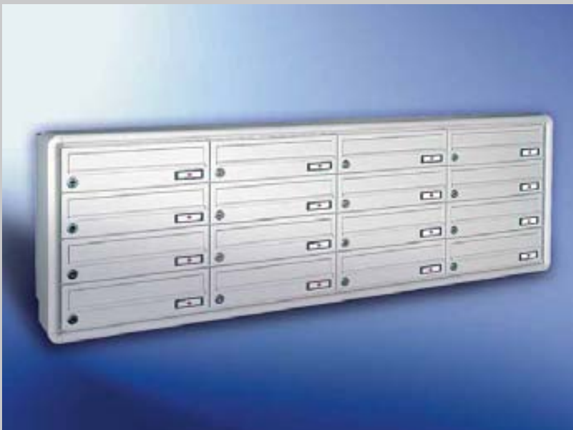
Fig. 19/3 Box format 370 x 110 x 270 mm, RS4000 casing for use when partially setting the unit in to the wall. Letter plates 335 x 33 mm.
