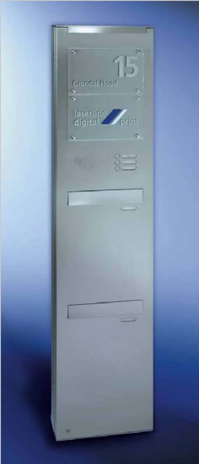
Fig. 29/1 V4A stainless steel pillar shaped mail box, two-part slide-through mail box unit with RSA , inclined opening 335 x 50 mm, box size 335 x 550 x 140 mm, rear removal door 335 x 440 mm bottom hung with two opening restrictors, fitted with LED lighting, 335 x 215 mm plexiglass panel for engraving as required, pillar height 2000 mm.
