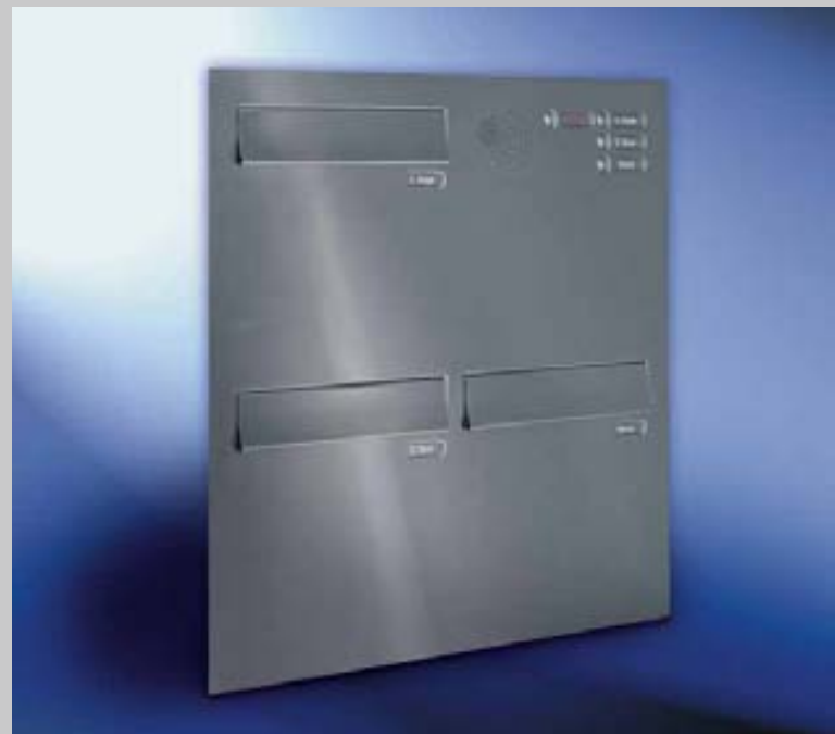
Fig. 23/4 Box format 370 x 330 x 145 mm, with RS50 , 24 mm front plate, with thermal break for mounting in door profile, with RSA , completely manufactured from V4A stainless steel. Letter plates 335 x 50 mm.
