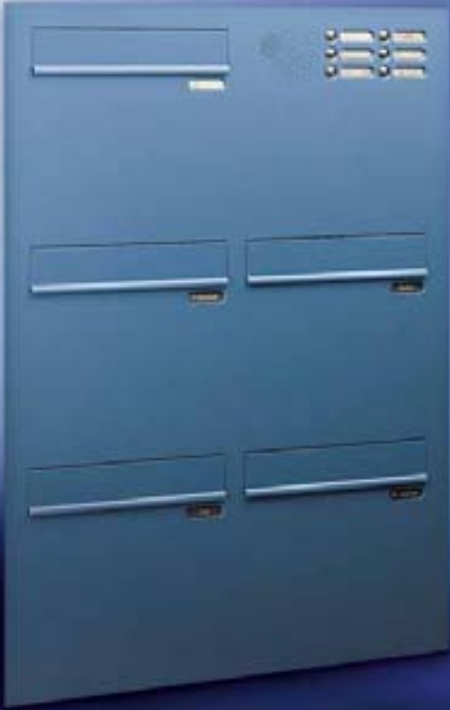
Fig. 22/1 Box format 370 x 330 x 145 mm, with RS50 , 24 mm steel front plate, with thermal break for mounting in door profile, with RSA . Letter plates 335 x 50 mm.
