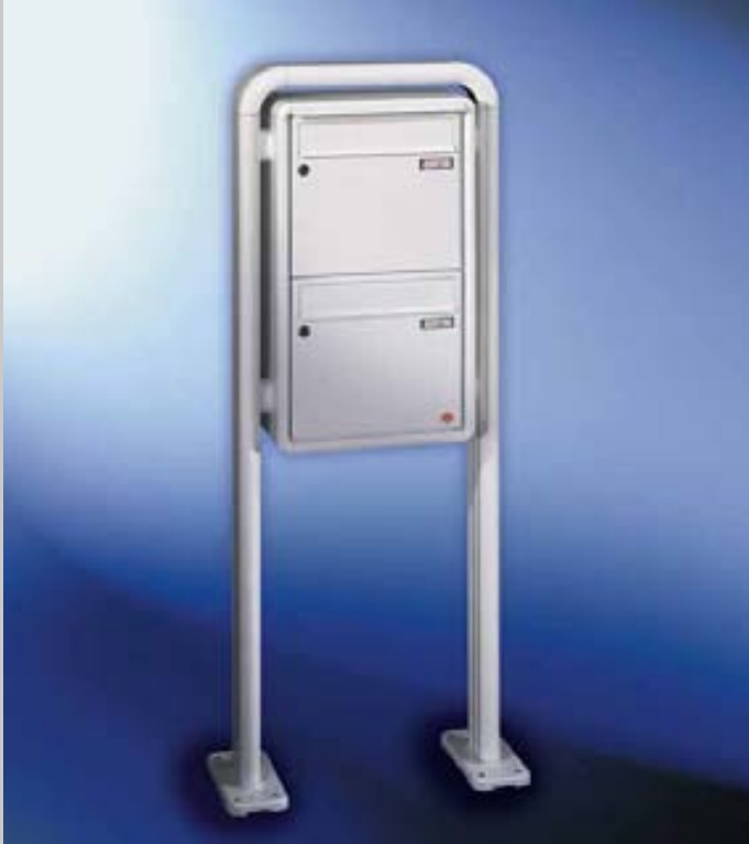
Fig. 13/1 Box format 370 x 330 x 145 mm, with RS50 , RS2000 aluminium casing profile and 105 x 45 mm oval tubular stand. Letter plates 335 x 50 mm
