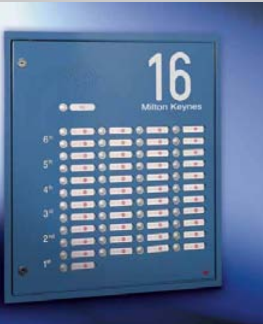
Fig. 32/1 Bespoke bell and intercom box with 20 mm aluminium plaster frame and RSA for flush fitting, with drop down front.
