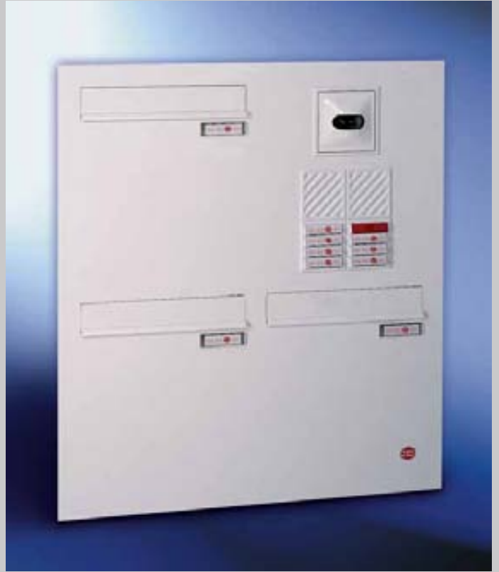
Fig. 22/2 Box format 300 x 330 x 100 mm, 24 mm aluminium front plate with thermal break for mounting in door profile, with metal mounting frame for CCTV camera supplied by others. Letter plates 265 x 33 mm.
