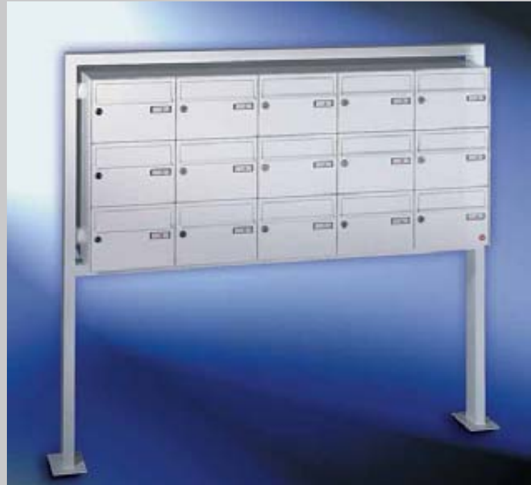
Fig. 17/2 Box format 300 x 220 x 385 mm with newspaper plate, sheet angular aluminium casing, and 80 x 40 mm rectangular tubular frame. Newspaper plate 265 x 50 mm.
