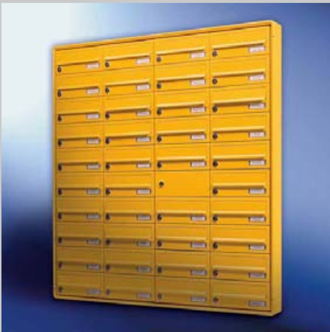
Fig. 38/3 Box format 260 x 110 x 385 mm, aluminium radius-profile main door frame. Front of the unit opens with 2 doors to allow mail to be inserted which is removed by the mail recipient having an individual key.
