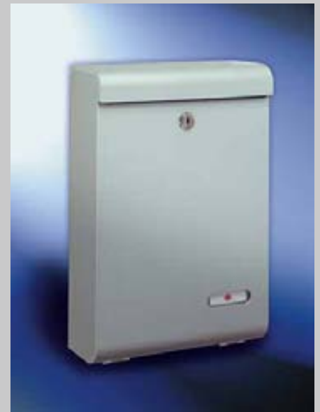
Fig. 35/6 Radio mail box, casing powder-coated sheet steel, tilting door and letter plate anodized aluminium EV1, RSA anti-vandalism name plate. Letter opening 230 x 33 mm. Box 270 x 405 x 118 mm.
