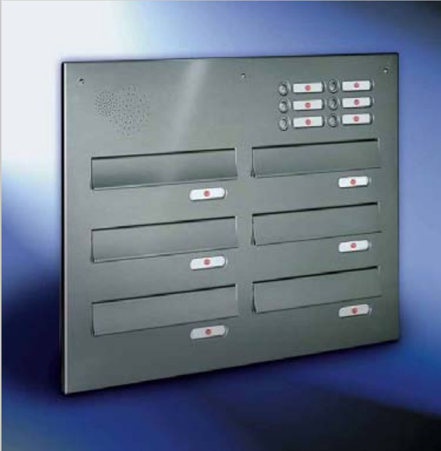
Fig. 27/1 Box format 300 x 110 x 265 - 410 mm, hinged V4A stainless steel front plate, with RSA . Letter plates 265 x 33 mm.
