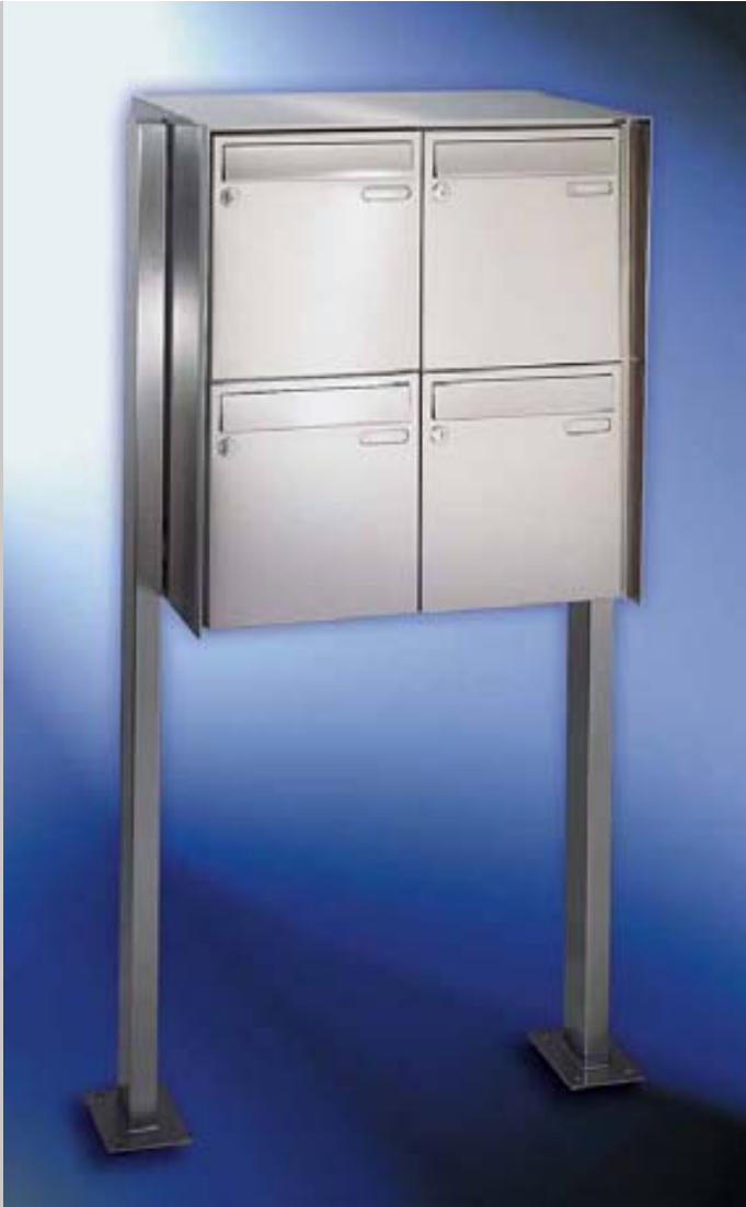
Fig. 17/1 Box format 300 x 330 x 385 mm, with RSA , angular casing with projection, and 80 x 40 mm rectangular tubular stand, completely manufactured from V4A stainless steel. Letter plates 265 x 33 mm.
