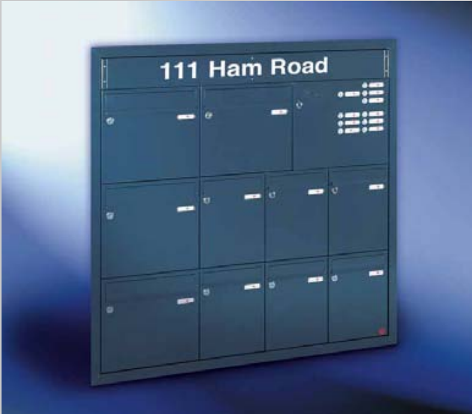
Fig. 11/1 Box format 260 x 330 x 100 and 370 x 330 x 145 mm with RS50 and RSA , bell and intercom box of special design, inscription box, 40 x 48 mm aluminium profile plaster frame. Letter Plates 230 x 33 mm or 335 x 50 mm.
