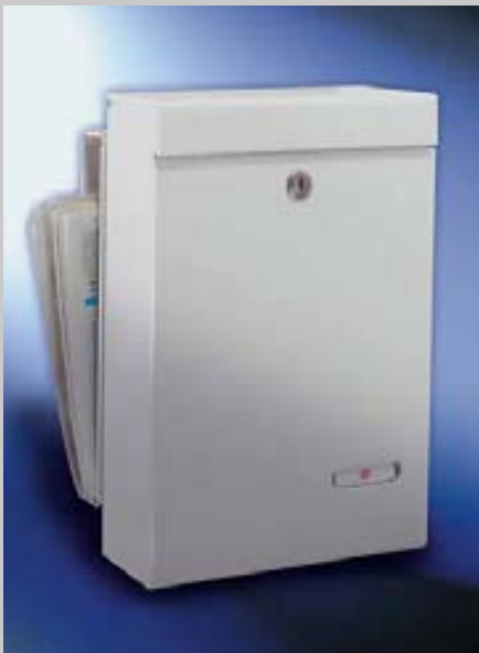
Fig. 35/4 Cubico mail box, casing profile, tilting door and letter plate powder-coated sheet steel, RSA anti-vandalism name plate. Photograph shows the optional newspaper box fitted behind the mail box. Letter opening 230 x 33 mm. Box 270 x 405 x 118 mm.
