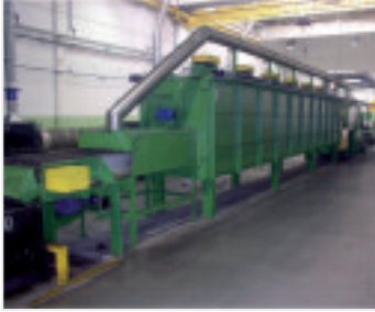
← Mesh Belt furnace line for hardening and tempering
