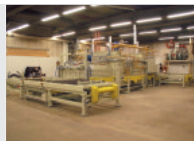
CuproBraz® 3-chambered furnace convection-fired →
