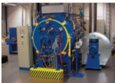
← CAB laboratory chamber furnace with vacuum purge
