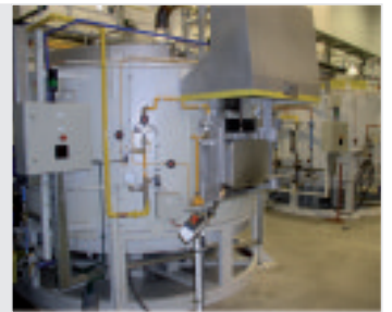
Rotary hearth furnaces for heating before forging →
