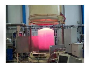
Coating of the heat-resistant elements of gas turbines
