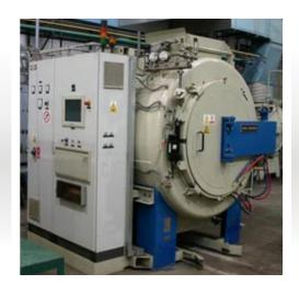
Vacuum furnaces for tempering and zero flow nitriding – cost effective nitriding with low emmissions
