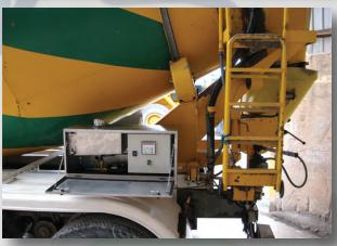
The digital interface allows the operator to dispense a controlled dose of additive into the mix.
