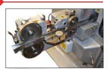
The 'Super 42HS' is a high-speed cut and wrap machine, which has been designed for strength and durability, as well as ease of operation and low maintenance. The machine sizes, shapes, cuts to length and wraps, toffee, chewy candy, bubble gum or high boiled sugar. The machine produces square, rectangular, or cylindrical shaped sweets. In the case of the 'Super 42CW' this usually a round shaped sweet in the "whirl" ("kiss") style.
