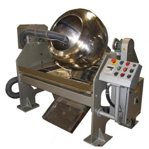
Conventional rotary pans are extremely versatile and can be used for coating and polishing a wide range of products such as nuts, dried fruit, licorice centers, jelly beans etc, using chocolate masses or sugar solution coatings.
