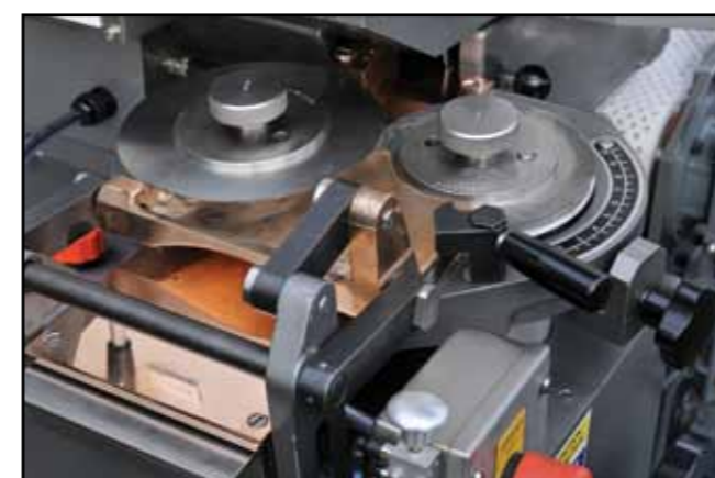
The speed of the candy rope is adjustable relative to the speed of the die
