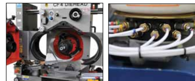
The use of clamps and slides allows the die to be quickly installed or removed
