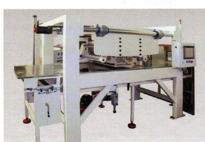
(48 on each) and retained by two keep plates. Pistons can be disconnected and easily removed for cleaning by lifting the keep plates and extracting them through the drive bar. Each drive bar is supported on bearings by two shafts to ensure a horizontal movement throughout the piston stroke.
