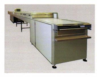
A 21 Meter cooling tunnel is provided as standard length can be varied if required.
