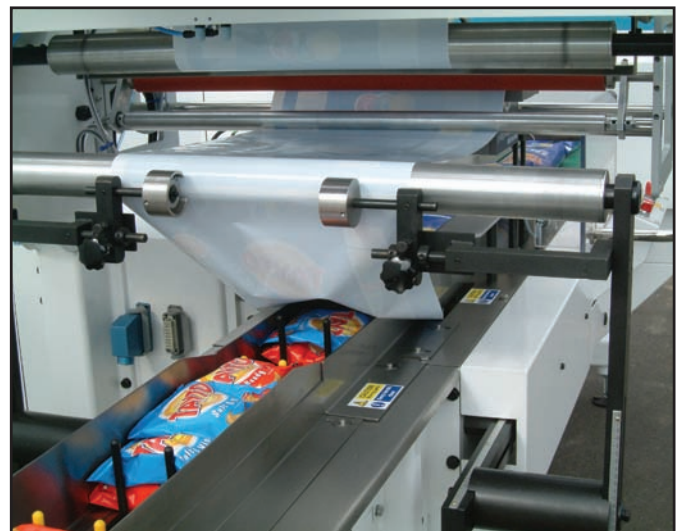
The infeed conveyor can be manually or automatically loaded
