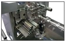
The NR10 has been developed specifically to wrap small square and rectangular chocolates in fold wrap style.
