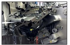
The products are manually placed onto the stainless steel infeed tray, usually from a plaque. They can alternatively be fed from an automatic belt conveyor system fed directly from the moulding plant, via an aligner-feeder belt system.
