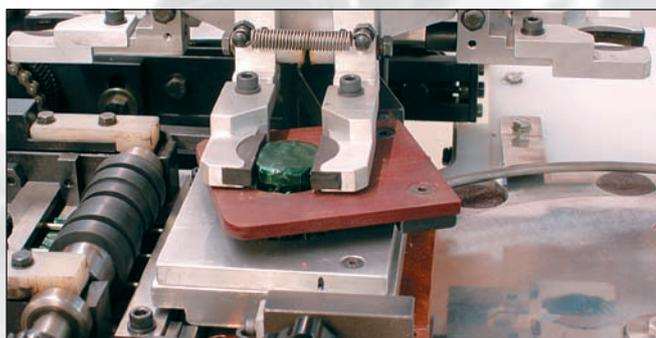
around the product. As the product is elevated through the brush, the wrapping wheel arms grip the sides. As the wrapping wheel rotates, the foil is tucked underneath the product by two tuckers to complete the wrapping.
