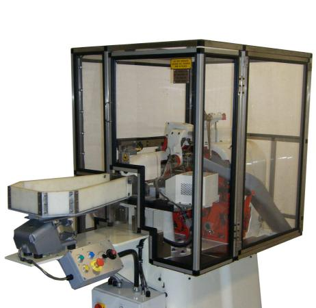
The 22B is primarily intended for twist wrapping sweets, lollipops or similar tablets, but other styles of wrap can be produced with the aid of attachments. It is in fact, a well proven and universal machine for the confectionery trade, being rapidly interchangeable for different sizes of sweet or style of wrap. It is gentle in action so that very highly filled pieces can be wrapped without risk of cracking or breaking. A special version is available for foil wrapping suppositories.
