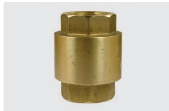
YORK check valve. Valve nylon with rubber seal. Stainless steel spring. Avoids backflow in any position. 12 bar
