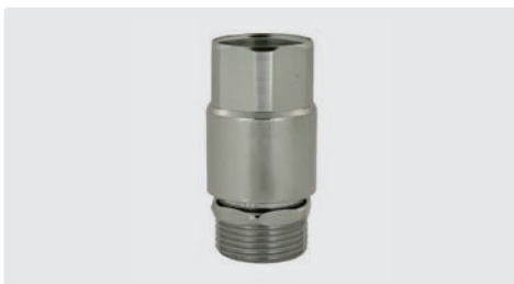
Chrome-plated brass. Backflow preventer according to DIN 19884 and DIN EN 1717. Avoids that cleaning agents come into the potable drink circuit in case of excess pressure in the water pipe. Required when direct connection to pump
