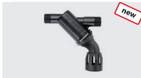
This is a special safety device that prevents water flowing back to the source, isolating the drinking water supply network from the circuit that supplies water to the cleaner. According to EN 60335-2-79: 2010. Max. 35 l/min. Min. 1 bar / max. 10 bar
