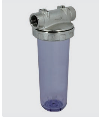
3-pieces. With drain. Head nickel-plated brass. Housing plastic. Max. 10 bar / 40 °C
