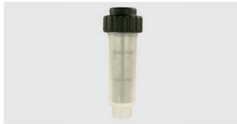
Complete with filter fine core washable (stainless steel and plastic). 50 microns. Max. 6 bar / 60 °C / 50 l/min
