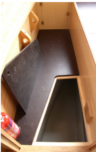
Access to the dry storage space next to the engine-hatch in the bulkhead above leads to the stern tube greaser and fuel tank valves.
