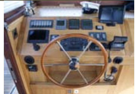
Comprehensive helm station, with demister system for windows, as well as electronic engine management system and bow CCTV camera.
