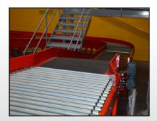
Roller conveyors can also be integrated into existing systems and used alongside belt conveyors.
