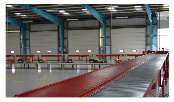
Fixed roller transport conveyors can be powered or gravity operated. These conveyors offer a low-cost solution to material handling or act as the perfect compliment to a larger system. Powered roller conveyors can be integrated with gravity conveyors and all other Sovex products.
