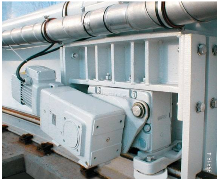
Architecture in motion with Demag travel units, consisting of an angular geared motor, integrated wheel block and guide rollers
