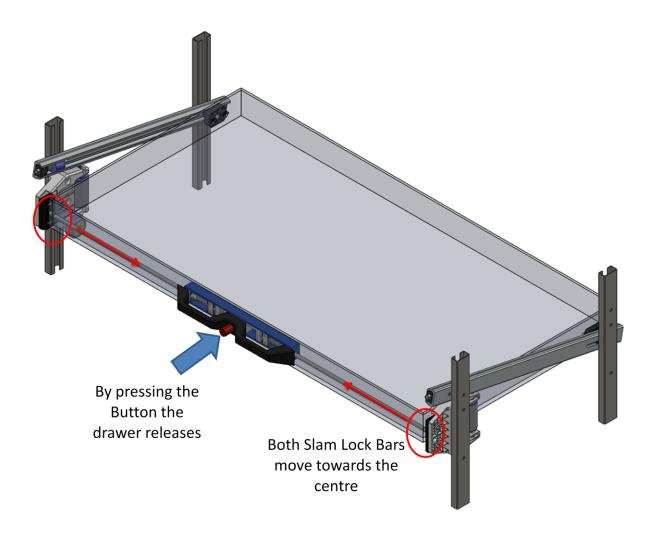
To open the drawer the operator presses the red button on the Front Handle.
