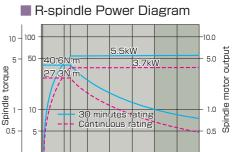
60 1,000 2,000 3,000 4,000 5,000 6,000 7,000 r/mir 1,269 Spindle speed Unusable range of ejector
