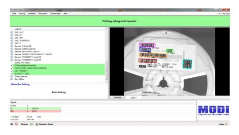
After applying the **customer-specific label**, the contents of the labels can — for additional security — be checked against the suppliers' labels in a further reading process.
