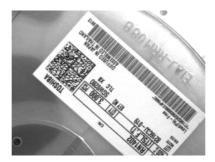
Using the label coordinates detected by the overview camera, the mirror is steered to the label to be read with millimetre precision so that the *ADOMO* camera can capture the label with the highest resolution.
