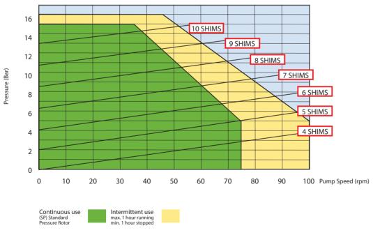
For product temperatures above 65°C and/or viscocity's above 2000 mPas use one shim less than shown
