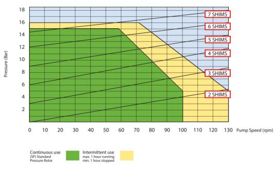
For product temperatures above 65°C and/or viscocity's above 2000 mPas use one shim less than shown.
