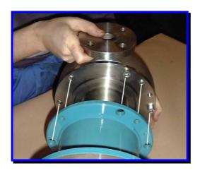
The casing/cartridge assembly can now be assembled to the pedestal (bareshaft unit) or the pedestal/motor assembly. The pedestal should be secured using the supplied fasteners with fastener anti-seize. The screws should be tightened to a torque of 40Nm (28.8 ft.lb).
