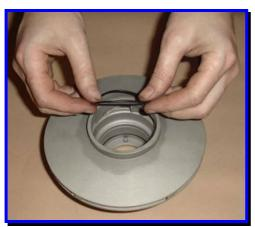
Front bearing o-ring kits are separated into the two common size o-rings. The smallest set is fitted into the external grooves in the backplate assembly shaft. The largest set is fitted into the internal grooves in the front of the pump shaft and the bearing holder.
