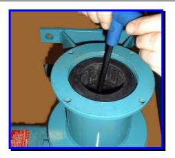
Any adjustments in outer magnet height by lifting or lowering the magnet assembly. When the setting distance is correct the screws are tightened. The magnet height is then to be rechecked.
