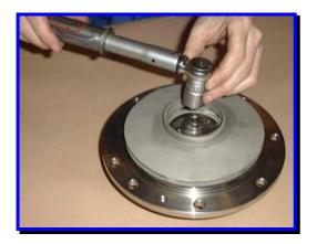
The locknut is then fitted onto backplate assembly onto the protruding shaft with fastener anti-seize.
