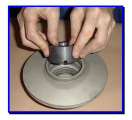
Note: Care should be taken not to damage any bearing components particularly when passing over anti-rotation pins. Any bearings damaged during fitting should be replaced prior to continuation of assembly.
