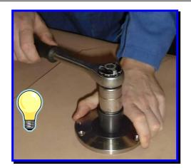
The supplied rear bearing washer and locknut is fitted with fastener anti-seize to the containment tube shaft once rear bearing thrust ring and sleeve are in place. The locknut should be tightened to a torque of 30Nm (21.6 ft.lb).
