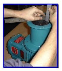
The outer magnet complete with taper lock adaptor and bush are then lowered onto the motor shaft. The outer magnet setting distance of 6mm, taken from the highest point on the magnet assembly to the highest point on the pedestal (see picture), should now be checked.
