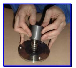
Bearing lubricant is applied to all surfaces machined with o-ring grooves.
