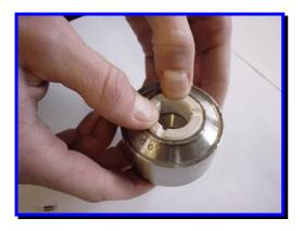
The single rear bearing component should be pushed into the rear of the pumpshaft. Care should be taken to ensure the hole in the bearing and the anti-rotation pin in the pumpshaft are correctly aligned.
