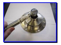
The impeller is fitted to the shaft and secured with the impeller locknut and washer using fastener anti-seize. The locknut should be tightened to a torque of 40Nm (28.8 ft.lb).
