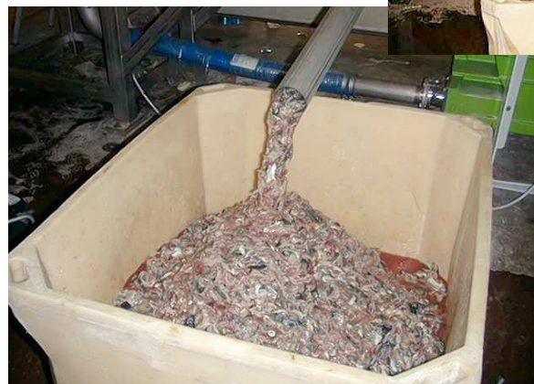
A Verderflex VF peristaltic pump transferring the fish slurry. The unit uses a positive displacement principle to move the slurry. A Verderflex pump can handle thick, viscous slurries, run dry and provide a powerful suction lift.
