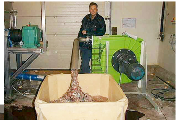
A Verderflex VF peristaltic pump transferring the fish slurry. The unit uses a positive displacement principle to move the slurry. A Verderflex pump can handle thick, viscous slurries, run dry and provide a powerful suction lift.
