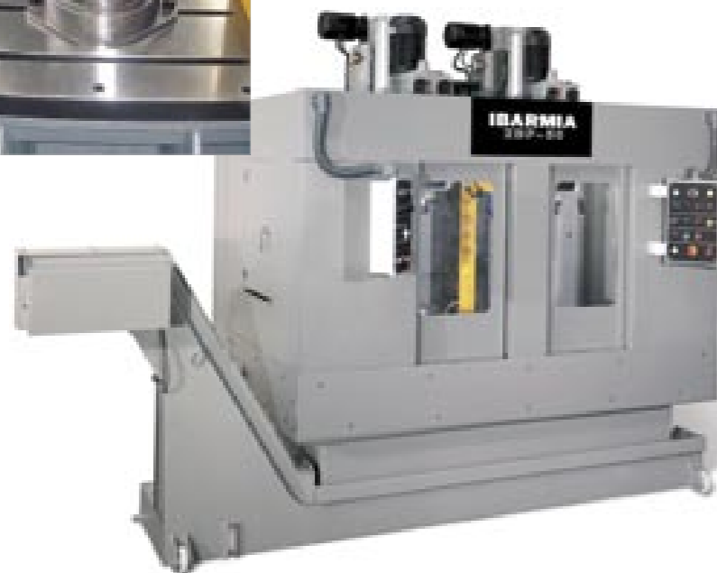
2 Headstock drill battery including full guarding, automatic doors, working area division, synchronized clamping tools, automatic chip conveyor and outside control panel.
