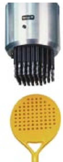
Simultaneous drilling of 76 holes in a paddle pallet.
