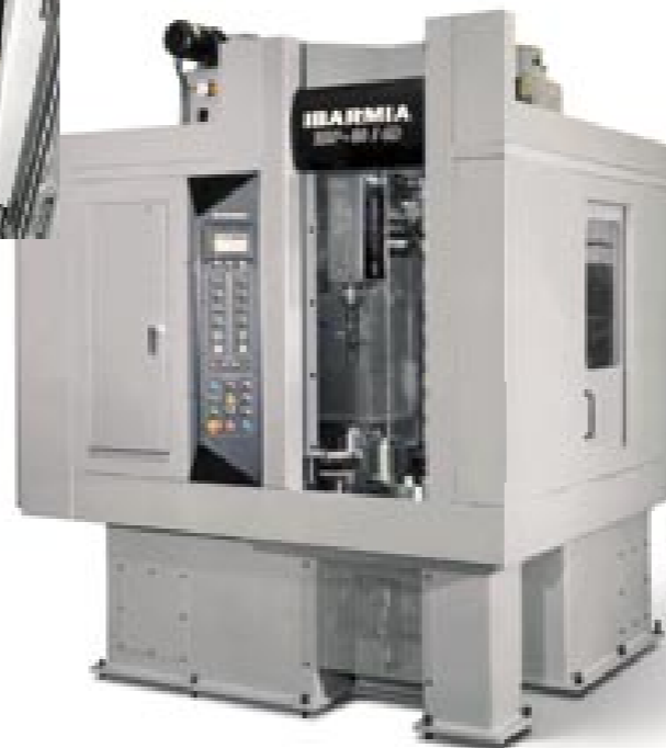
4 Position circular drill battery: • Position 1: loading with automatic regulation of the piece length. • Position 2: drilling operation. • Position 3: tapping operation. • Position 4: automatic ejection of the pieces to the basket.
