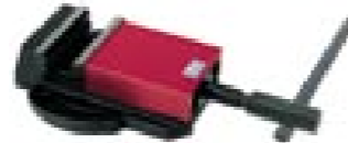
FL-116 Vise with fixed base. Maximum opening: 116 mm. Jaw width: 100 mm. Jaw height: 31,5 mm. Net weight: 9 Kg. Available for Z/X/A/B/C series.
