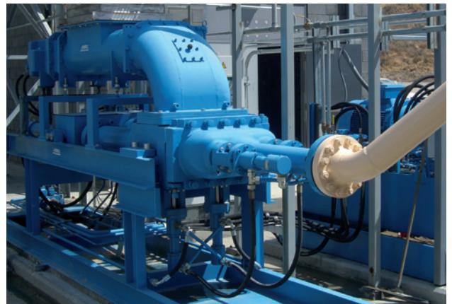
ABEL SH with double screw feeder for transfer of dewatered sewage cakes
