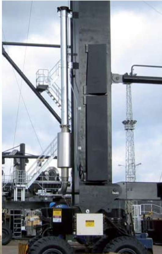
DOC Diesel-Oxidation Catalyst PM 20-30% reduction
