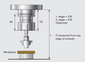
The two-stage displacement travel in the Z-direction (optional), with its maximum displacement, permits machining with high tools or angle units without any problem, even in the case of thick workpieces.
