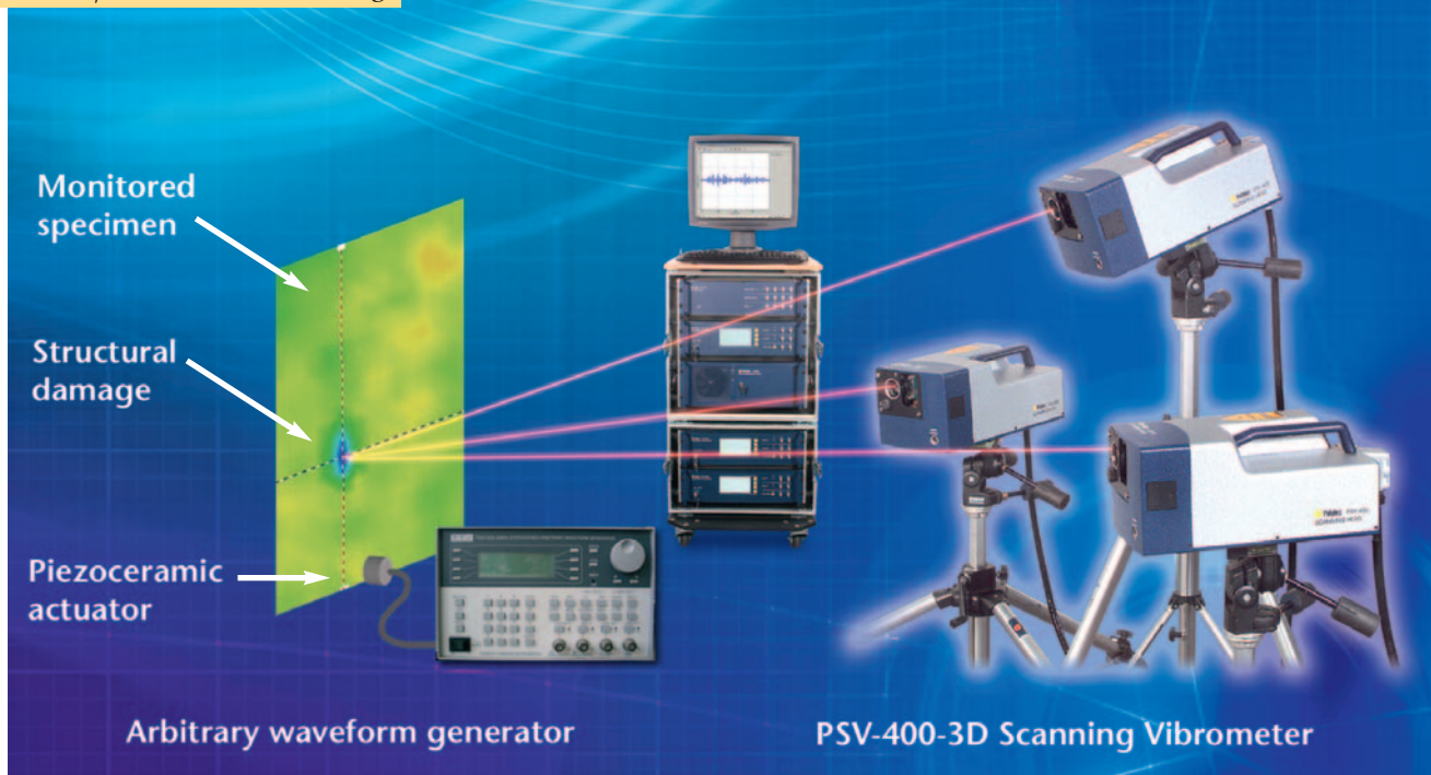
Figure 1: Experimental arrangements for Lamb-wave damage detection using 3-D laser vibrometry as a receiver.
