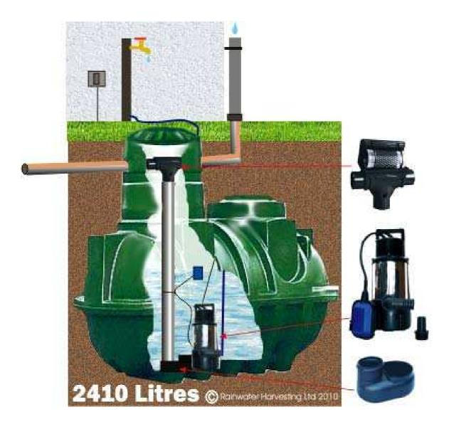
The "T" shaped item is the in-tank/in-line/compact filter.
