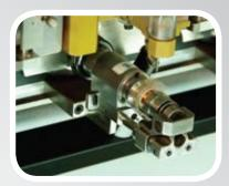
Much of our production uses fully automated processing and many of our wide range of machines are microprocessor or computer controlled. These automatically wind, bond, solder, lead cut and terminate during the winding cycle. Universal winding facilities for small and medium size batches are available on various types of single spindle machines that require a minimum of tooling and setting-up costs. Batches of 10 - 60,000 units per week are typical production runs.
