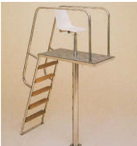
R.765 Pedestal Observation Chair 100mm diameter stainless steel single column, for grouting into pool surround, 38mm diameter handrail ladderway with treads, swivel plastic seat, non-slip platform.
