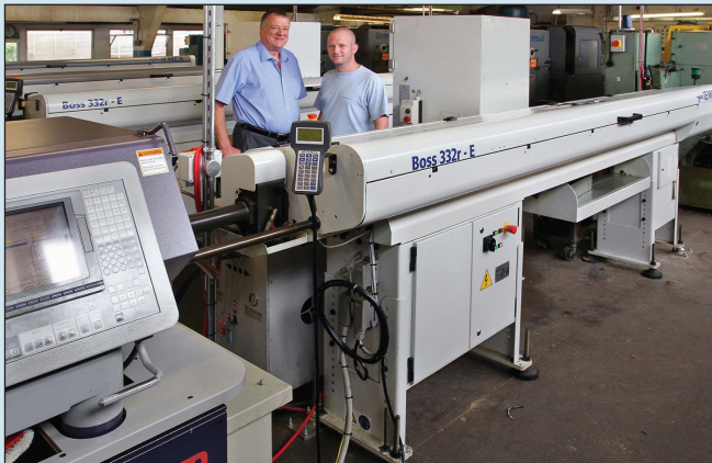
Iemca Boss 332r-E bar magazines fitted to Citizen M32 sliding-head lathes at Precision Products, Rustington. Managing director Brian Owen is pictured left.
