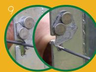
Push the wire in the slot, then down past the keeper
