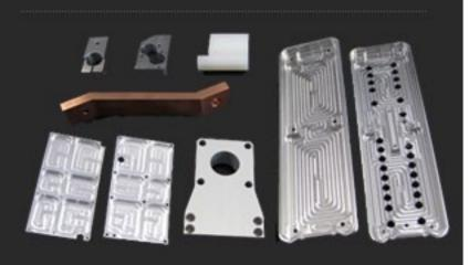
A wide range of CNC and conventional machined parts produced from billet materials.
