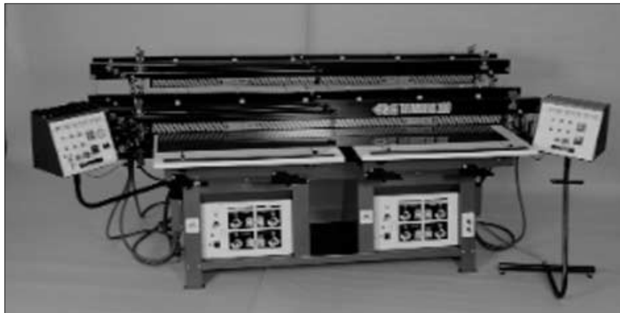
Figure 19 Line bending machine
