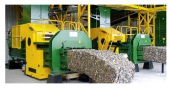
The material, which is delivered to incineration plants for energy production, must be baled for efficient handling, storage and transport.
