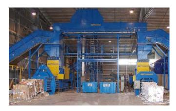
Two new balers were purchased for the plant, one LP 100 DH4S and one LP 140 XH2S with a feed opening of 1100 x 2250 mm. The LP 140 XH2S has a combined press force of 210 tons, a bale format of 1100 x 1100 mm and 2 x 75 kW electric motors. This giant presses everything from cardboard to shredded industrial waste and produces up to 50 tons or over 800 cubic meters per hour.
