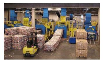
this flow, the plant is equipped with 6 fully automatic balers from Presona in sizes varying from 40 to 100 tons press force. There are also two Presona perforators for mechanical perforation of PET bottles – a quarantee for obtaining maximum bale weight.
