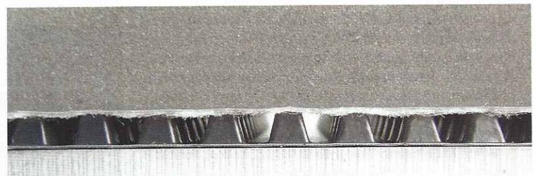
Figure 4 Soft/hard platen test and cusped geocomposite at 35kPa
