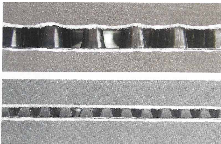
Figure 3 Soft platen test and cusped geocomposite drainage sheets at 35kPa
