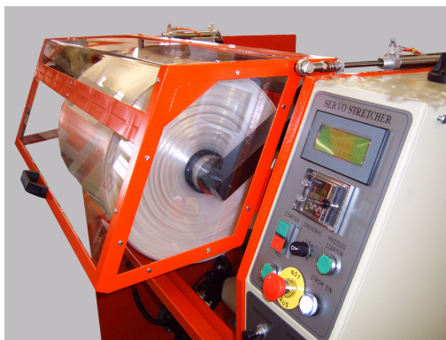
Heavy duty rewind max capacity 460mm.
