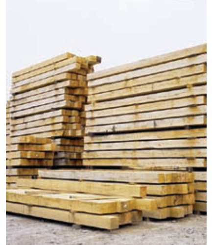
Fresh sawn oak beams
