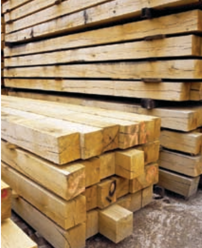
Fresh sawn oak beams
