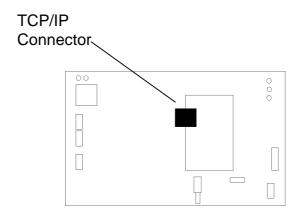
The TCP/IP connection supports Ethernet 10/100 Base-T. The connector sits underneath the LCD and is best accessed by following the procedure:
