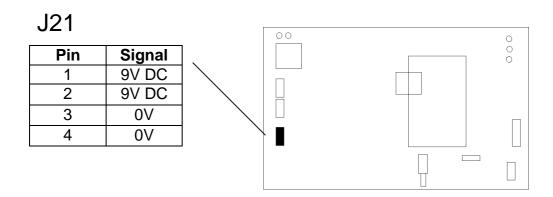
**Note:** The power connector on the HRX3000 is on the left hand side of the unit, whereas on the HRX5000 the connector is on the right. In both units the power connector is adjacent to the regulator heat sinks.
