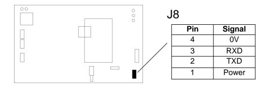
**Note:** Pin 1 on J8 is at the bottom of the HRX3000 **Note:** PC cable is the same as for the HRX5000
