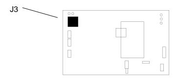
The unit can accept a plug in Modem which sits on the underside of the main PCB. The footprint is compatible with a PSTN landline modem or a GSM radio modem. To access the modem:
