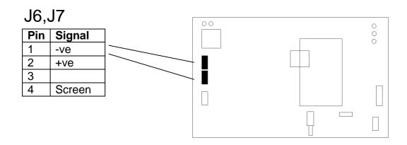
A Master HRX3000 is able to communicate with up to 15 Slaves over a twisted pair RS-485 bus. Two connectors are fitted in each terminal to make wiring easier in the field.
