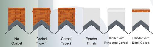
Our brick clad chimneys are manufactured using bricks from site and are supplied ready for pointing on site for a perfect match.
