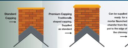
Our brick clad chimneys are supplied with a Premium capping. Standard capping or supplied ready for mortar flaunching on site are optional.
