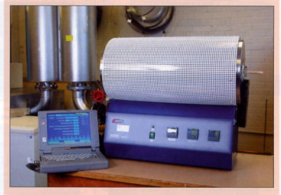
This 1200°C, three-zone horizontal tube furnace from Elite Thermal Systems is said to be providing big benefits at the Corus Technology Center - Swinden Laboratory, where it is being used to simulate manufacturing conditions on newly developed grades of steel wire. Previously this research was carried out in two tube furnaces, but a lack of temperature uniformity over the heated length meant that the results obtained could become unreliable.
