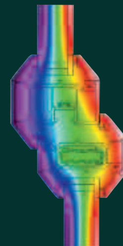
Thermal transfer through Liniar 'A Rated' sash/transom
