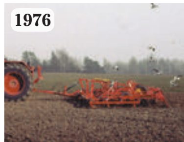
1976 In 1976, boundaries were moved with SH-2, a 14.8 m wide harrow for very large farms.
