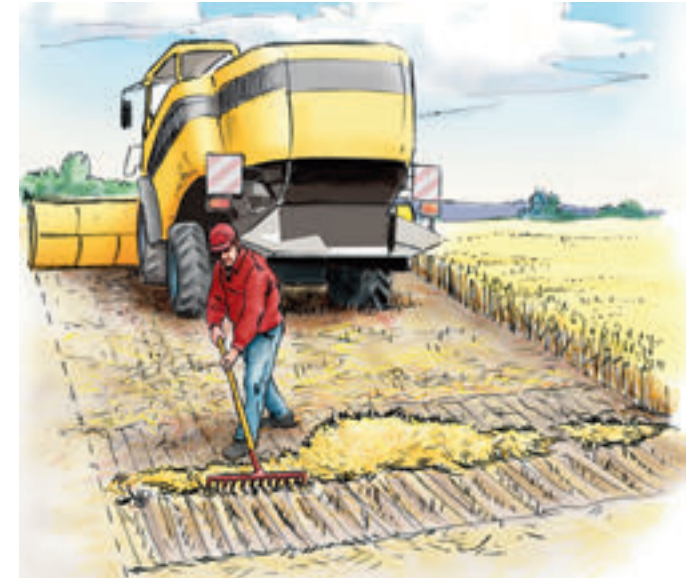
To test whether you have good straw distribution after the combine harvester, simply rake together a 1 m strip across the entire width of the combine and check to see if the density of the strip is even.
