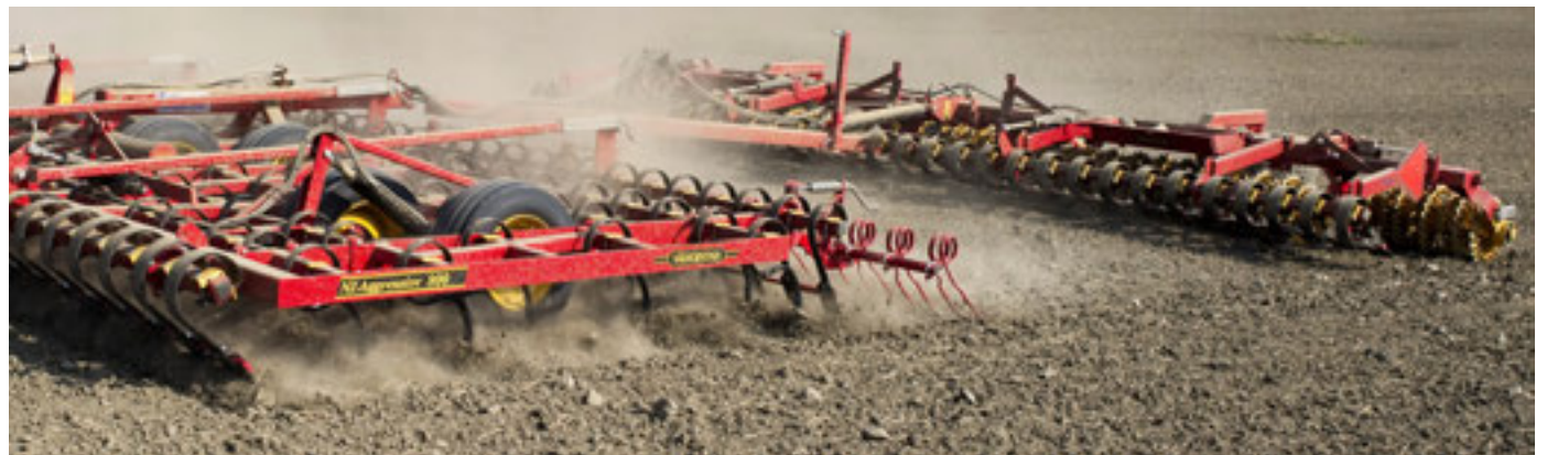
A following Crosskill roller ensures level consolidation after NZ Aggressive.
