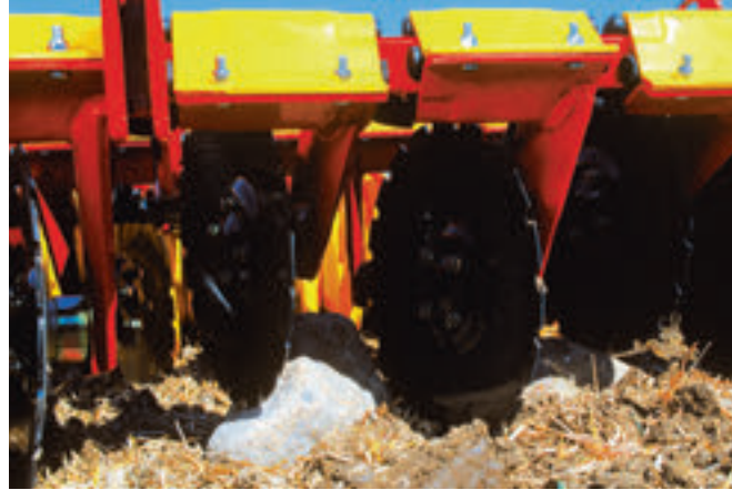
The discs are individually mounted in maintenance-free rubber cushioning. This improves the precision at depth and laterally which in turn extends disc life.
