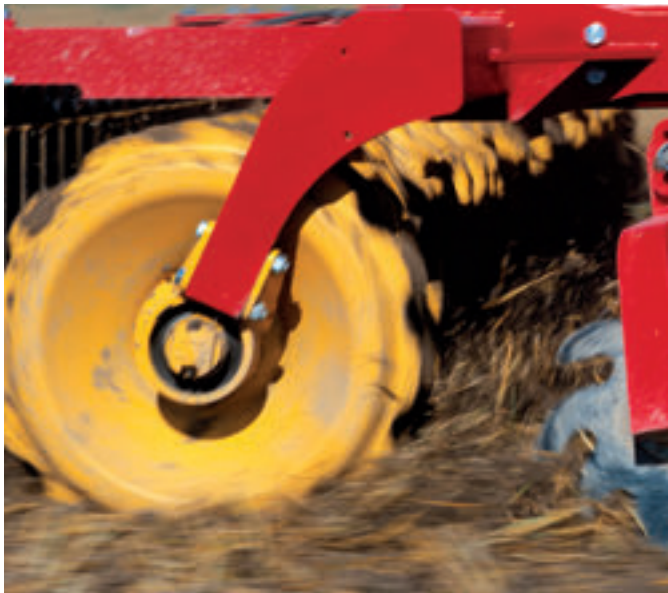
The steel roller breaks up straw lying near the surface and presses it into a shallow soil layer in order to achieve an optimal decomposition rate.
