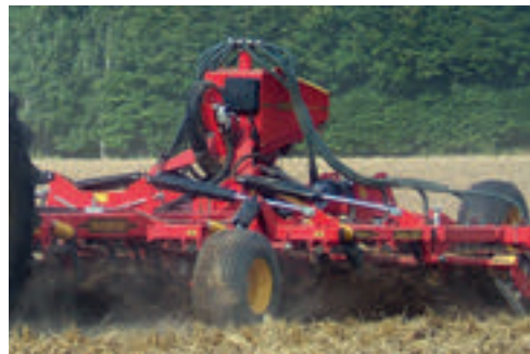
BioDrill 360 with pneumatic seed hopper is intended to be fitted on the larger Cultus models.
