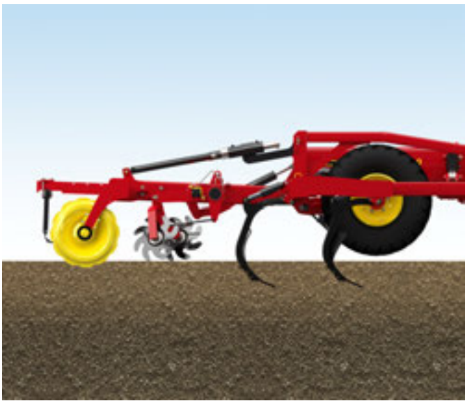
In dry conditions, the entire weight of the machine can be carried on the roller.
