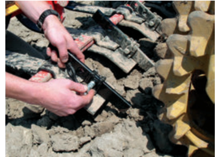
Knife tools can be fitted quickly and without the need for tools, thanks to Quickchange.
