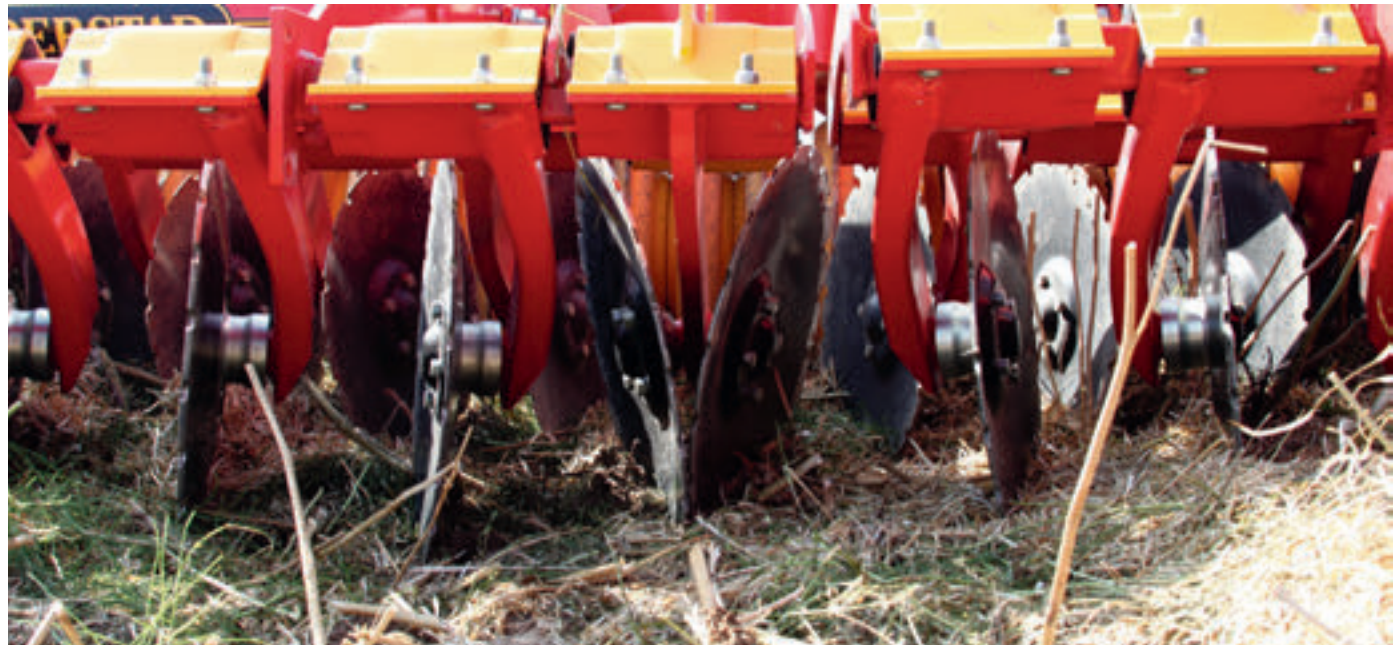
The discs are positioned in an X-shape, ensuring that the machine runs straight behind the tractor. This is essential when using GPS and to avoid overlapping.
