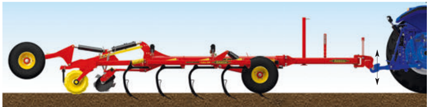
With the hydraulic arm drawbar well adjusted, the draught requirement is lowered.
