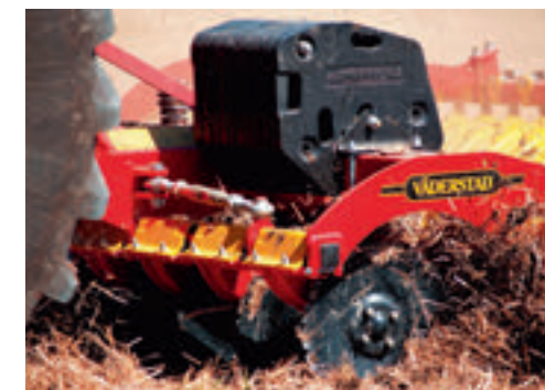
Extra weight package of 400/800 kg available as option for Carrier 300-400
