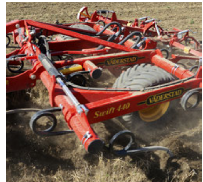
Swift 400/440 has extra wide 520 mm carrying wheels for a stable ride even at high speed on cloddy soils.
