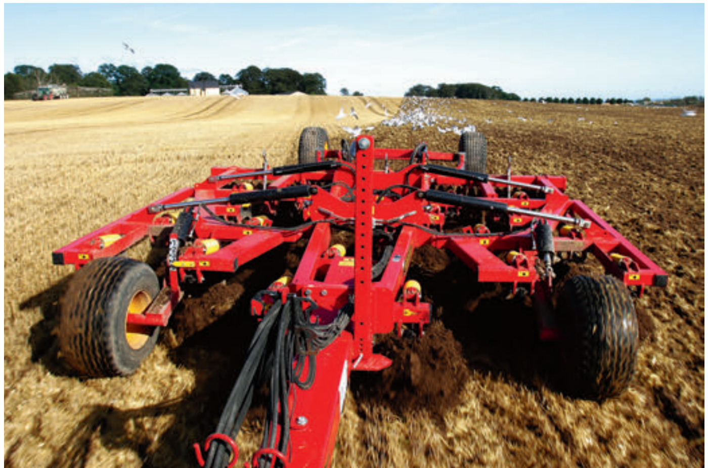
It is easy to optimise cultivation depth hydraulically from the cab. This is essential for good cultivation on fields with varying soil type.
