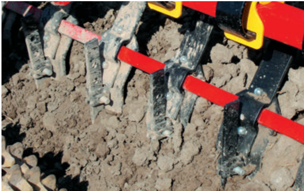
Crossboard with a stabiliser bar makes the roller an effective cultivating implement.
