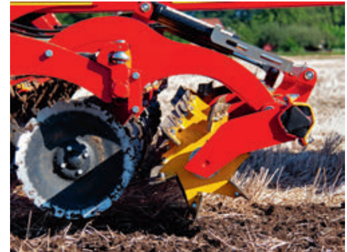
Crosscutter is controlled hydraulically from the tractor cab.
