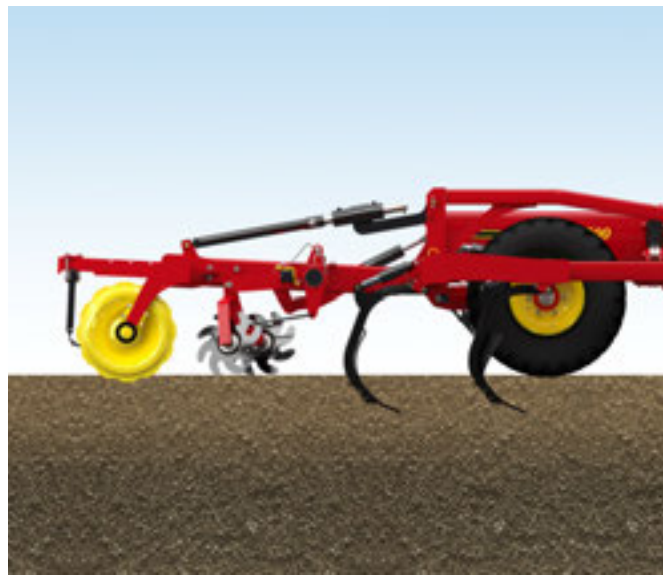
On lighter soils, the roller is raised so that it just runs on the surface.
