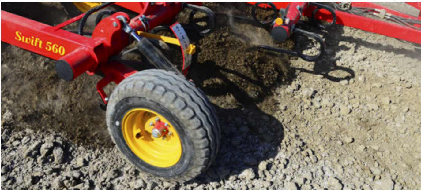
Swift 560 is equipped with fixed support wheels with hydraulic setting from the cab as standard.
