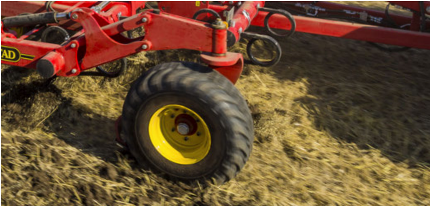
Swift 560 has the option of large pivoting support wheels. These support wheels are controlled hydraulically with a master/slave system. Swift 720 and 870 are equipped with large 520/50x17 support wheels as standard.
