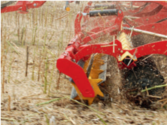
Crosscutter creates a false seedbed and efficiently chops up harvest trash.
