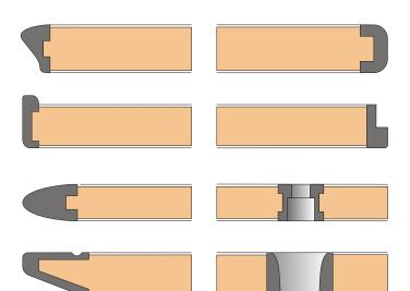
Casting can create special details like recesses for inserts and grommet edgings as well as varying profiles on each edge of a single top.
