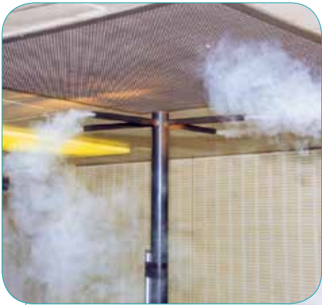
Left: Flow visualisation of moderate wind speed with no evidence of any "short circuiting" of the air movement
