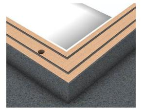
Figure 3 - Silicone placement
